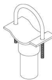
FIG. 882 PIPE SADDLE SUPPORT WITH U-BOLT PAGE 103
